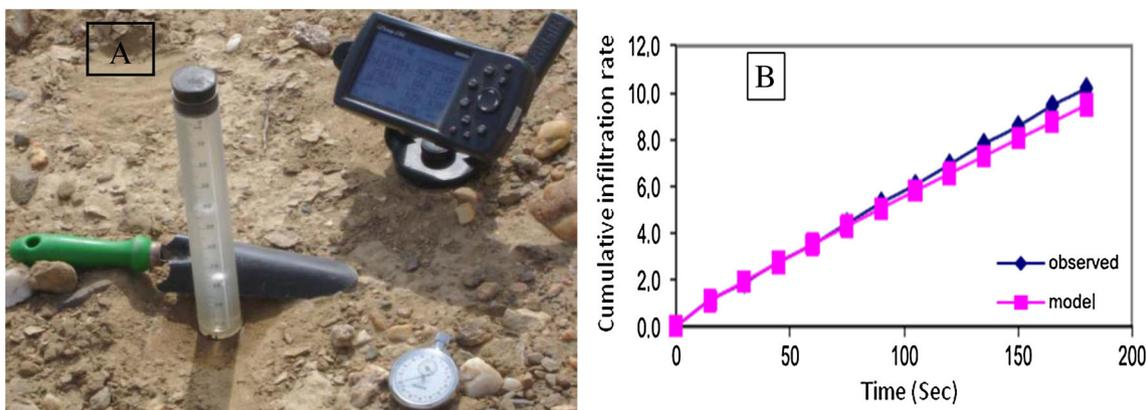
**Fig. 5** Field infiltration test. **a** Field photograph showing the disk infiltrometer. **b** Example of cumulative infiltration rate for non-cultivated coastal plain soils
