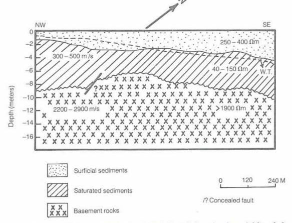
Fig. 9. Generalized subsurface geological section. Geological boundaries are based on resistivity and seismic velocity constrasts.
