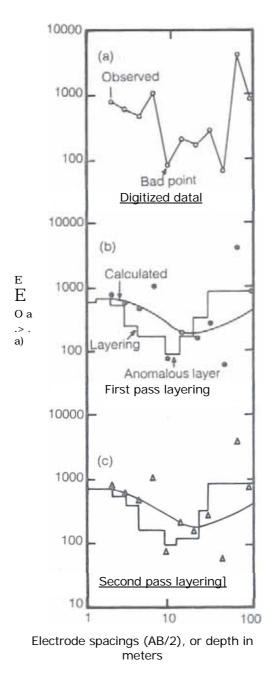
Fig. ,6. Automatic interpretation of VES 2: (a) digitized curve, (b) first-pass results with anomalous layer and poorly-fitting calculated curve, and (c) second-pass results with anomalous layer eliminated and calculatzd curve still not closely matching the observed curve.
