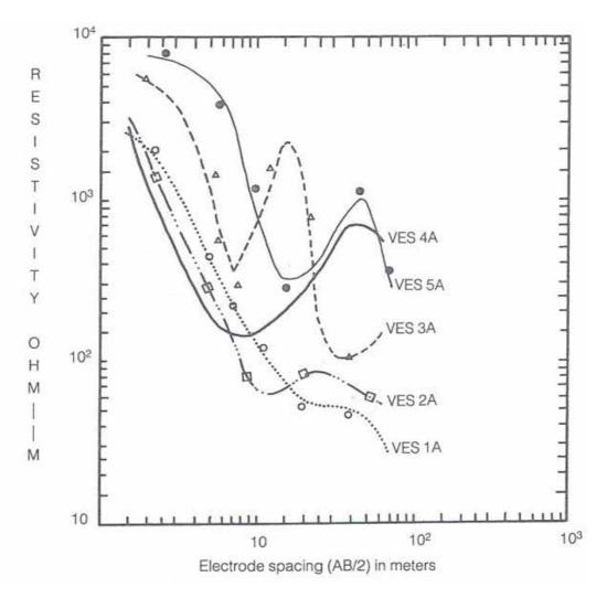
Fig. 4 Six VES curves with electrode spacing (meters) versus apparent resistivity (ohm-m) obtained along a traverse perpendicular to the trend of wadi Bisleale.
