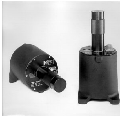
Figure 2x. The SS-1 seismometer (vertical and horizontal components)
