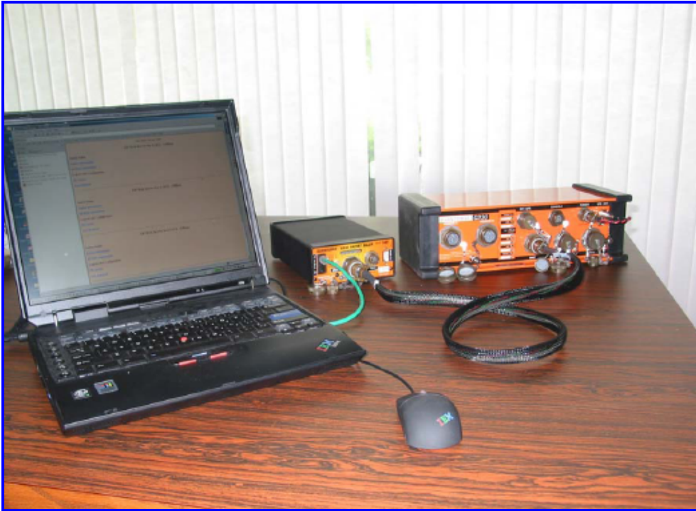
Figure 5x, shows a general view of the Digitizer Q-330 and the external storage Baler while configuration at the lab. After configuration and testing all units then the system is disassembled again and packetized to be moved to the field sites.
