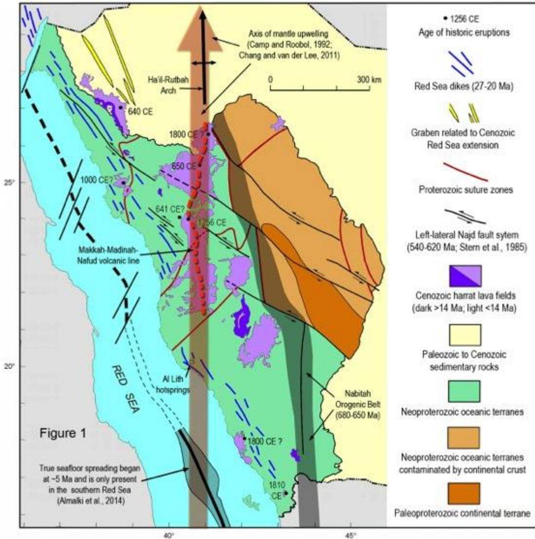
**Figure 1.** Regional map of tectonic, lithostratigraphic, and magmatic features of western Saudi Arabia. Note axis of volcanic activity that diverges from the trend of the Red Sea. The axis intersects a series of north-west trending faults and presumed zones of weakness that may control magmatic activity and enhance shallow permeability below the volcanic cover.
