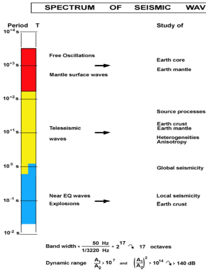
**Frequency range, bandwidth and dynamic range of modern seismology and related objects of research. The related wavelength of seismic waves vary, depending on their propagation velocity, between several meter (m) and more than 10,000 kilometer (km). The amplitudes to be recorded range from nanometer (nm) to decimeter (dm).**
