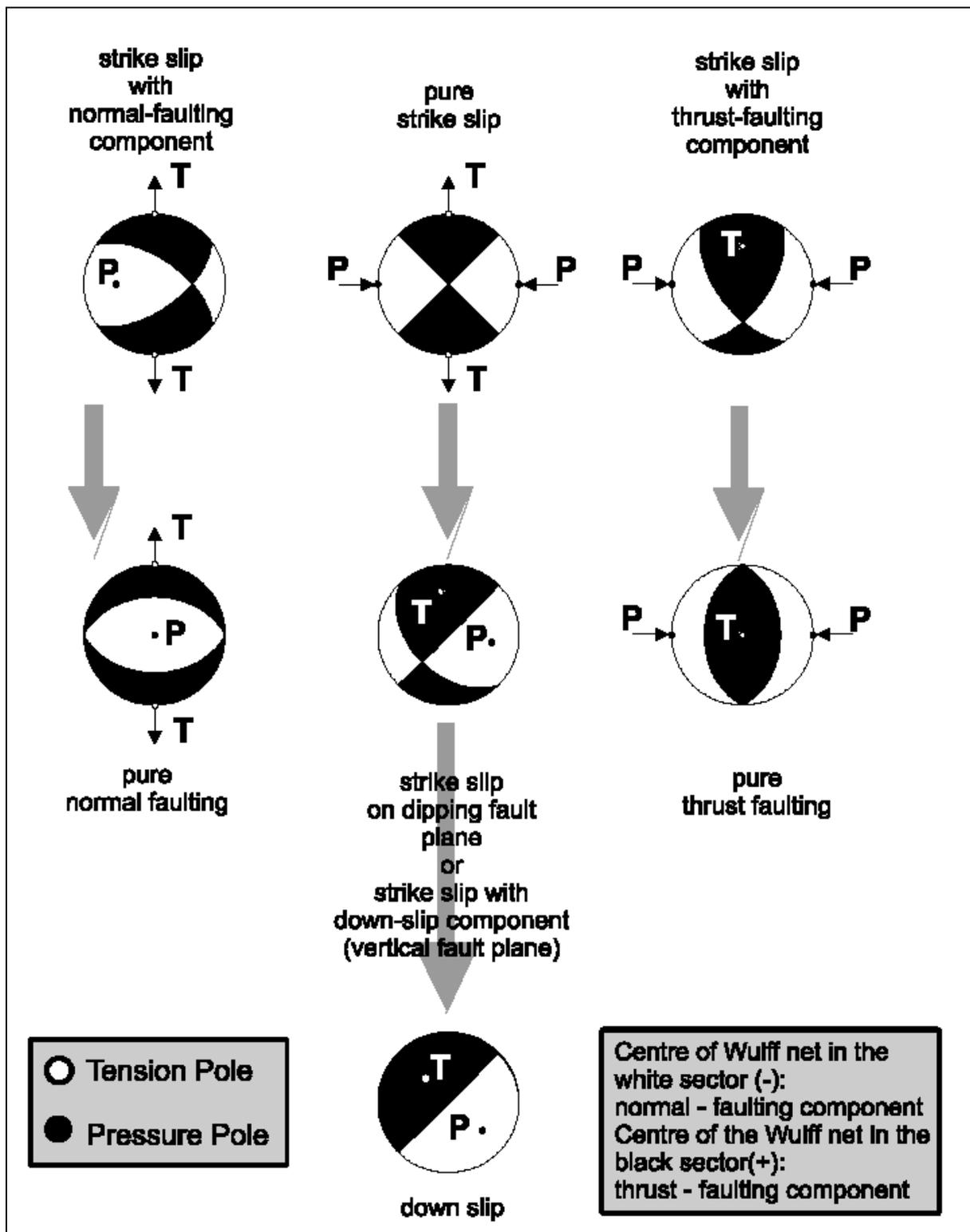
Beach-ball. presentation of the net projections of the fault plane cut-traces and of the penetration points (poles) of the P- and T-axes through the lower focal hemisphere for different faulting mechanisms. White sectors correspond to negative and black sectors to positive first-motion polarities.
