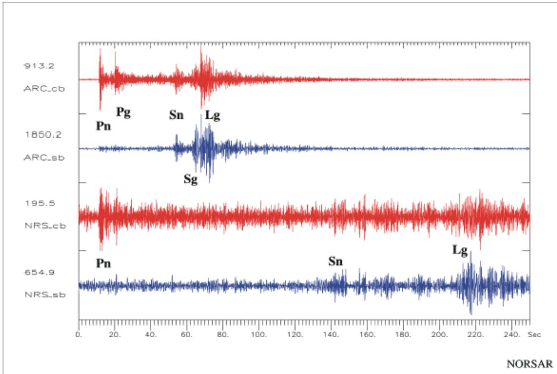
**Records of Lg, together with other crustal phases, in records of a Kola peninsula mining blast (MI = 2.4) at the Norwegian array stations ARCES (distance  $D = 391$  km; upper two traces) and NORES ( $D = 1309$  km, bottom traces). cb and sb . P- and S-wave beams of the vertical elements of the array, filtered with 2-8 Hz and 1-4 Hz, respectively.**
