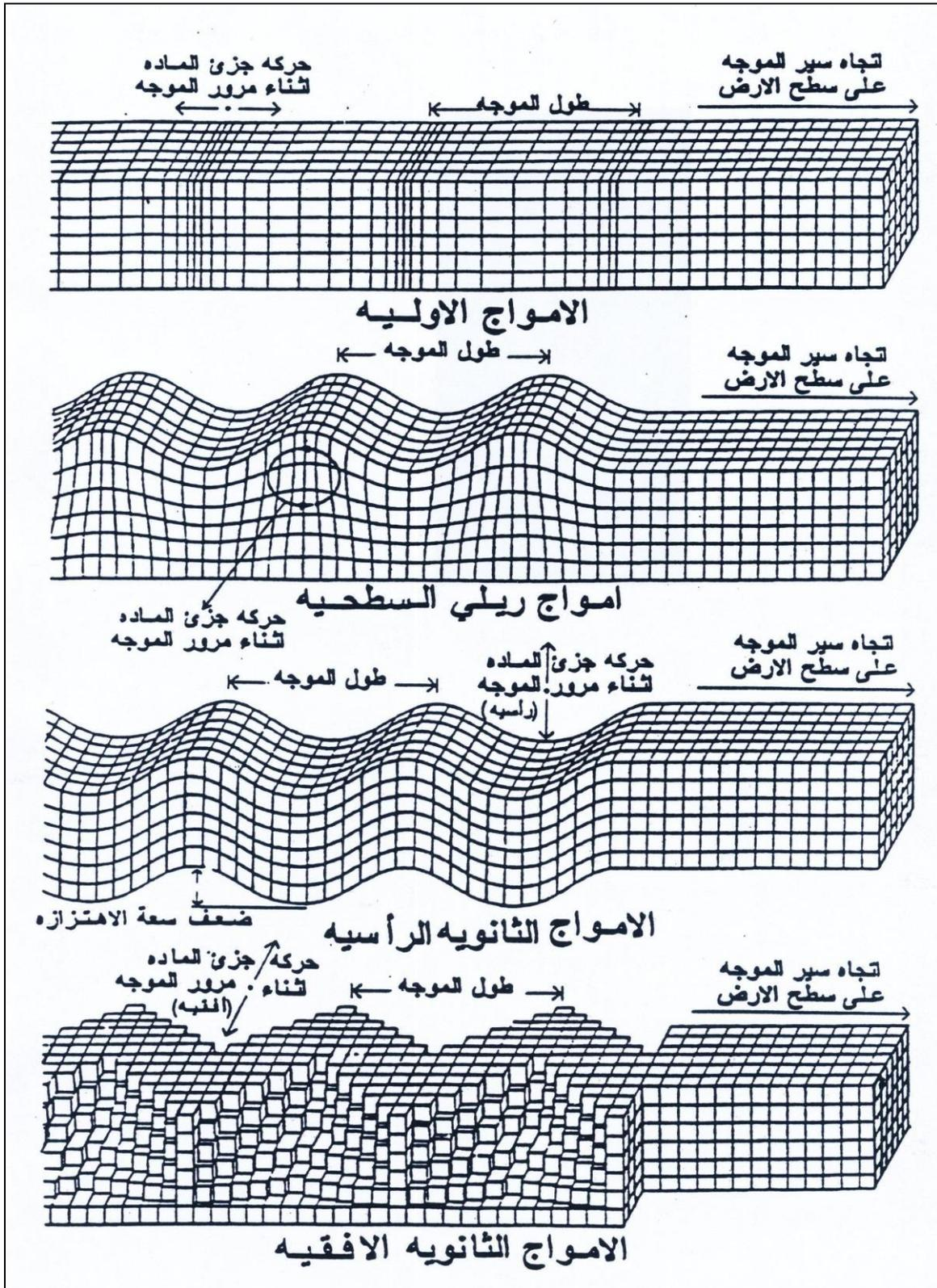
Fig. 2 :Types of seismic waves : Primary, Secondary and Surface waves
