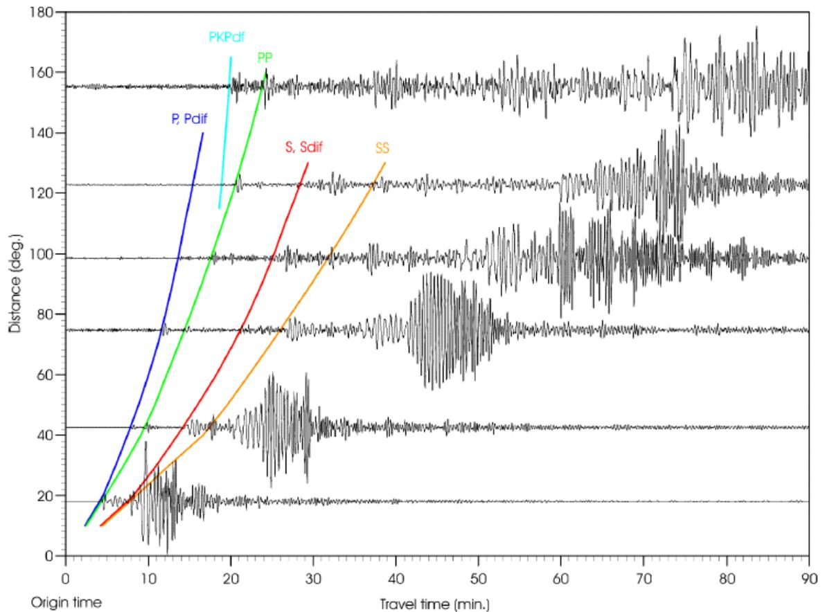
**Long-period filtered vertical-component broadband records of station CLL, Germany, of shallow earthquakes in the distance range  $18^\circ$  to  $157^\circ$ . Note the strong later longitudinal (PP) and transverse energy arrivals (S, SS) that are recognizable in the whole distance range, and the dispersed surface wave trains with large amplitudes. The record duration increases with distance (courtesy of S. Wendt, 2002).**
