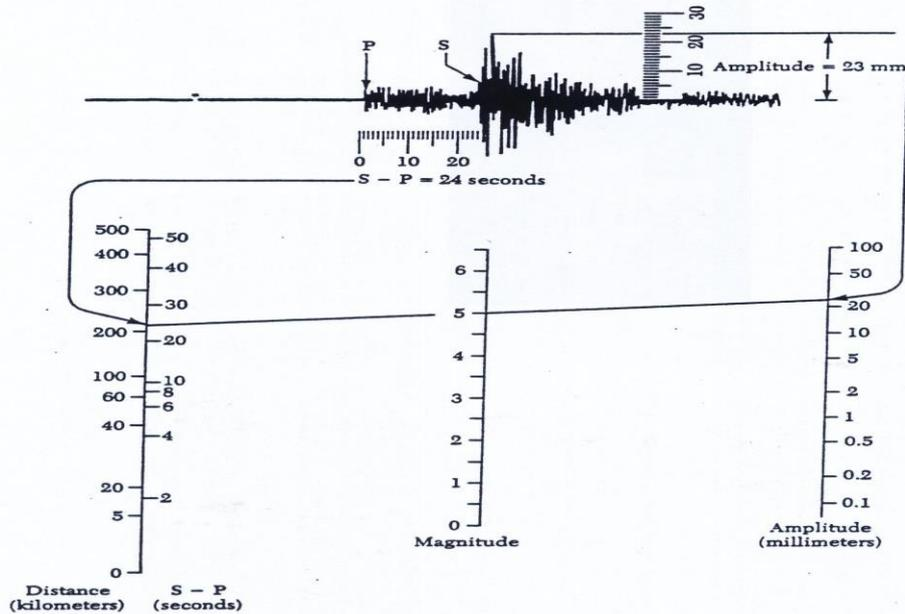
Procedure for calculating the local magnitude,  $M_L$
