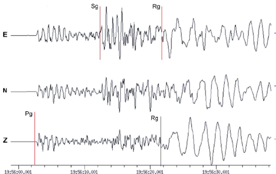
**Mining induced rock burst south of Saarbrücken, Germany, recorded at station WLF in Luxemburg ( $D = 80$  km,  $h = 1$  km, MI = 3.7). Note the strong dispersive Rg phase.**
