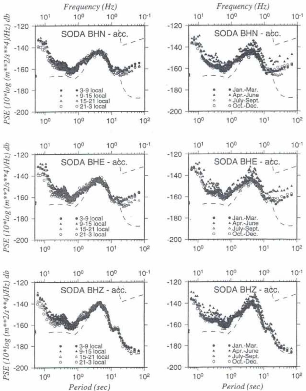
Figure 7. Diurnal and seasonal variations at SODA station. Axes as indicated in Figure 5.
