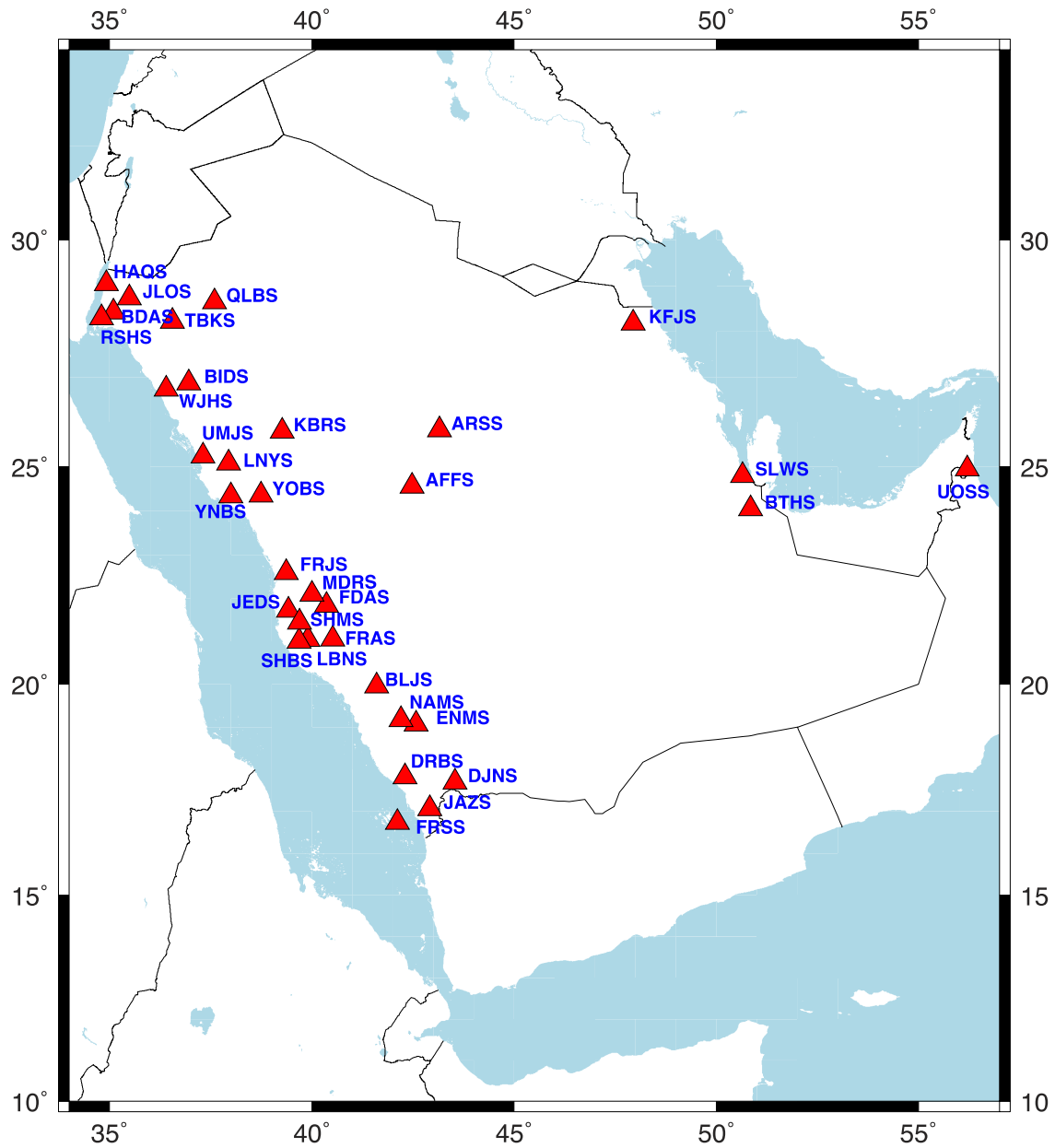
Figure 4.6. A station map showing the broadband seismic stations across the Peninsula used in the ambient noise correlation. Note: additional stations included to expand coverage, but off this map are FURI, ANTO, ABKT, GNI and KIV. (Data courtesy Saudi Geological Survey (SGS), King Abdulaziz Center for Science and Technology (KACST) and Incorporated Research Institutes for Seismology (IRIS/PASSCAL))
